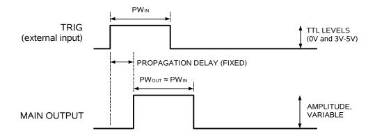
The delay, pulse width, and frequency (when in the internal mode), of the OUT pulse can be varied with front panel controls or via the GPIB or RS-232 computer interfaces.
