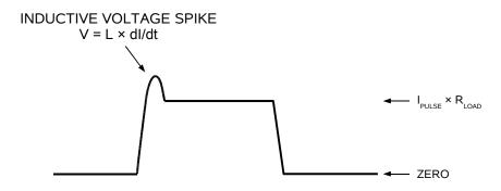
Attaching a current transformer (for measuring current waveforms) can add significant inductance, because of the necessary wire length that must be fed through the transformer. The Pearson 2878 requires approximately 1.5", and the 410 requires 3". Both will degrade the output current rise time.
