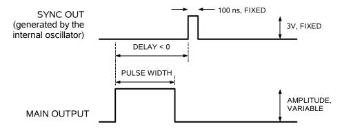
The next figure illustrates the relationship between the signal when an external TTLlevel trigger is used:
