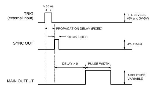
As before, if the delay is negative, the order of the SYNC and OUT pulses is reversed.
